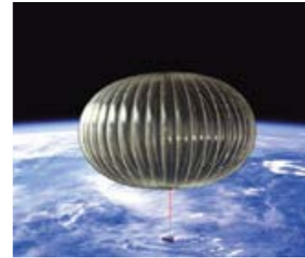
Artist's impression of a NASA superpressure balloon (at ~30 km altitude); they are regularly launched for earth observation and astronomy.
