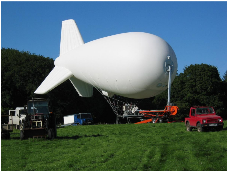
Figure 2. 15 metre diameter balloon test-bed.
