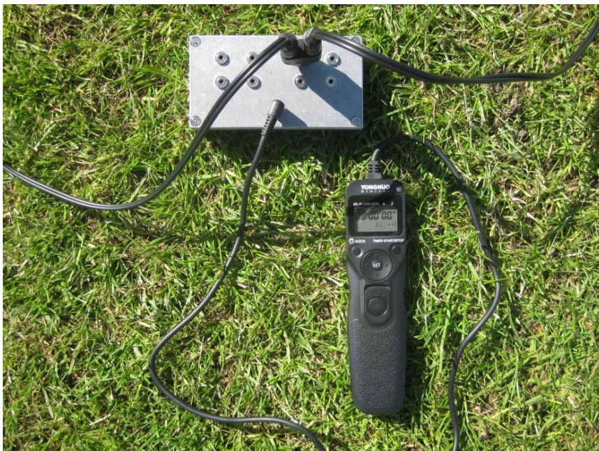
Figure 32. Intervalometer and junction box for synchronised triggering of cameras.
