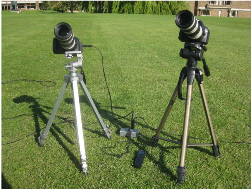
Figure 31. Stereo camera setup for outdoor kite testing.
