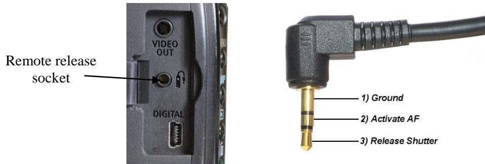
Figure 19. Remote release socket of a Canon DSLR camera and a 2.5mm jack for triggering the camera remotely.
