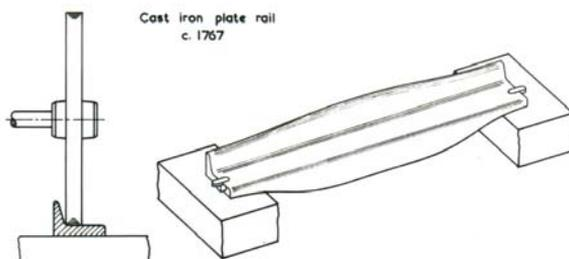
Original plate rails had vertical flanges to hold the wheels central
