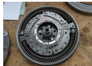
Fig. 2: (b) Gearbox side of automobile dual-mass flywheel with 4 bifilar pendulums
