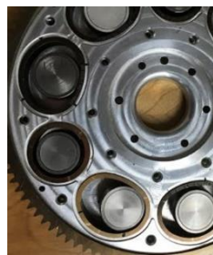
Figure 1: (b) Salomon or roller pendulums
