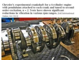
Figure 2: (c) Experimental automobile engine with bifilar pendulums
