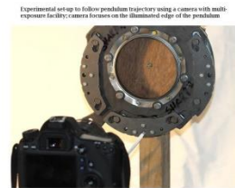
Figure 4: (b) Experiment to record the pendulum trajectory for a typical automobile bifilar centrifugal pendulum
