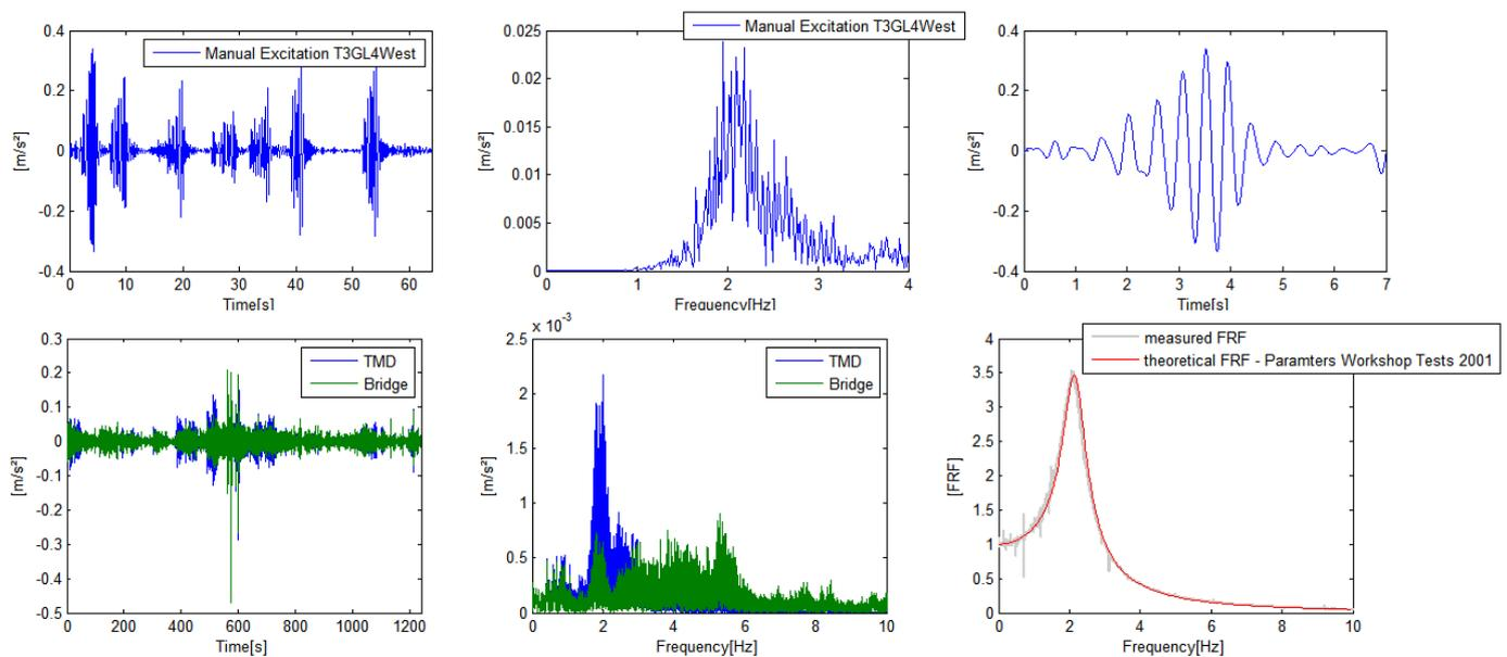
Figure 8: in-situ test results from the 2012 inspections, illustrating (above) the response of the absorber mass under direct manual excitation (time record, FFT spectrum and amplitude-time decay curve) and (below) ambient vibration records (time record, FFT spectrum and frequency-response function).
