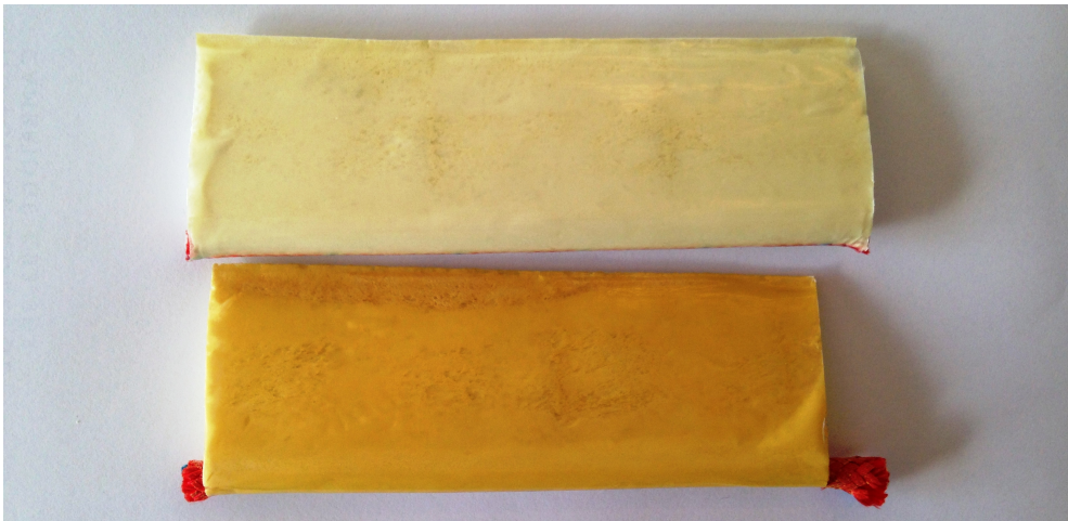
Fig. 6.24 Streamlined cable foam degradation to a brownish-yellow colour.
