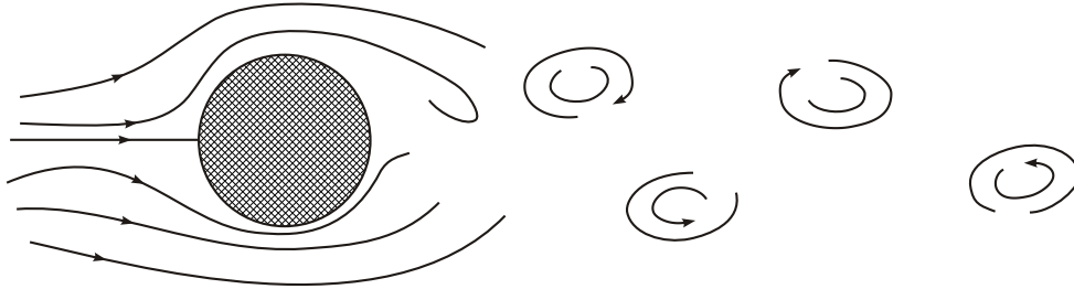
Fig. 2.14 Schematic of vortices generated by the sinuous instability of the wake behind a bluff cylindrical body in uniform flow [116].
