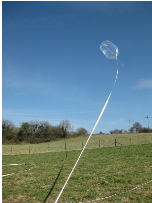
Fig. 6.18 Length of 50 m streamlined cable flown using a helium balloon in Somerset.
