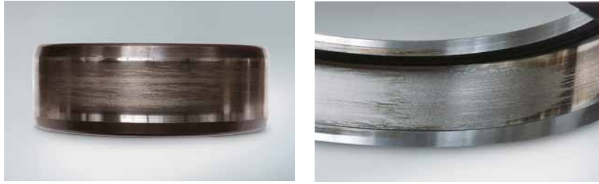
Figure 2.3: Typical smearing wear on bearing raceways. Source: NSK new bearing doctor catalogue [2] .
