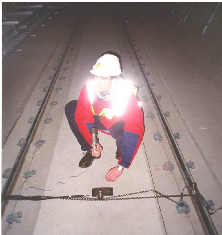
Figure 6.5: Photograph showing the use of the impulse hammer in conjunction with a rubber pad resting on the structure to be excited. Here the accelerometers are set out across the track.
