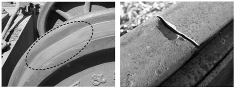
(a) Wheel flat (b) Uneven rail joint
