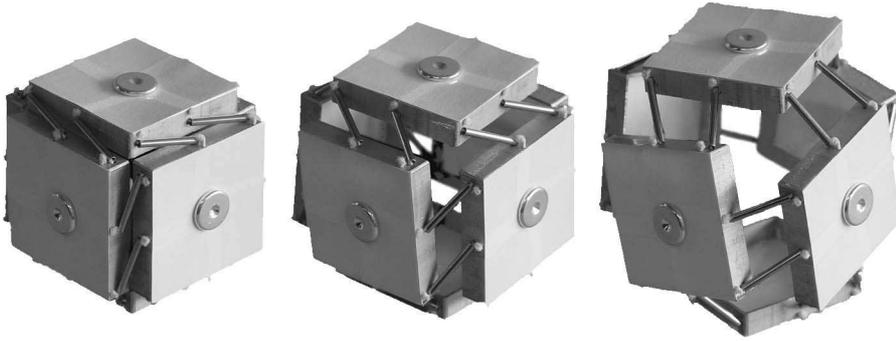
Figure 3. A double-link expandohedron based on the cube; the model is shown expanding from left to right. The faces consist of square-box sections; the linking bar is a tube containing a prestressed elastic string running face to face. The method of construction leads to the structure being most relaxed in its expanded state, from which it can be closed by drawstrings running between opposite faces. The drawstrings have been edited out of these images, for clarity.
