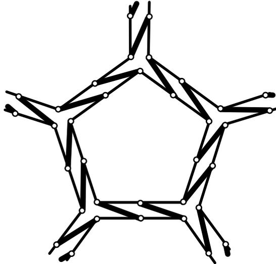
Figure 2. The construction of a double-link expandohedron around a regular pentagonal face. A simple arrangement, in which links run from vertices to edge mid-points, is shown; many other arrangements are compatible with the construction described in the text.
