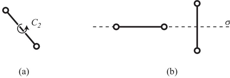
Figure 1: Possible placement of a bar with respect to a symmetry element in two dimensions, such that it is unshifted by the associated symmetry operation: (a)  $C_2$  centre of rotation; (b) mirror line.
