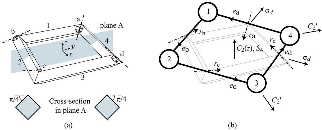
Figure 6: A spatial four-bar linkage. (a) The physical embodiment, showing four bars, 1–4, connected by four revolute joints, a–d. (b) A representation of the contact polyhedron,  $C$ , with the four bars shown as rigid bodies, connected by edges across the hinges. The axes of the revolute hinges a–d are shown as pseudo-vectors  $r_a$ – $r_d$ . Symmetry operations in  $G(C)$  are shown.
