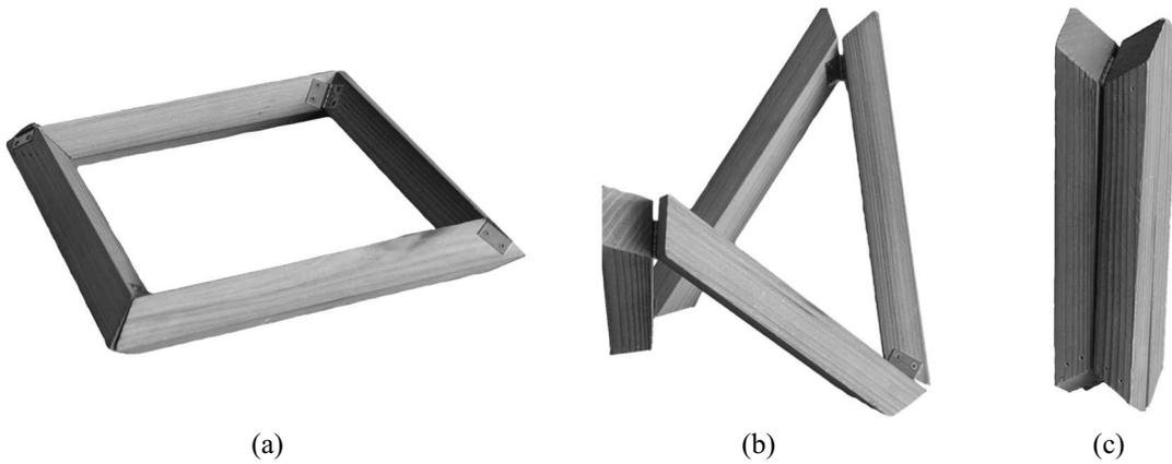
Figure 5: A spatial four-bar linkage, shown folding from its fully open state (a), to its fully closed state (c), where it forms a compact bundle of bars.
