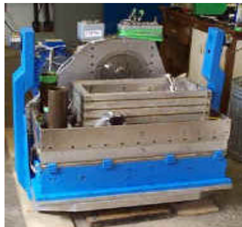
Fig.5 Self-contained swinging platform carries both the SAM actuator and the ESB soil model container
