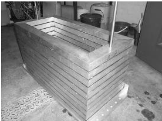
Fig.7 A view of the new large Equivalent Shear Beam (ESB) model container
