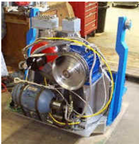
Fig.4 An overview of the Stored Angular Momentum (SAM) Earthquake Actuator
